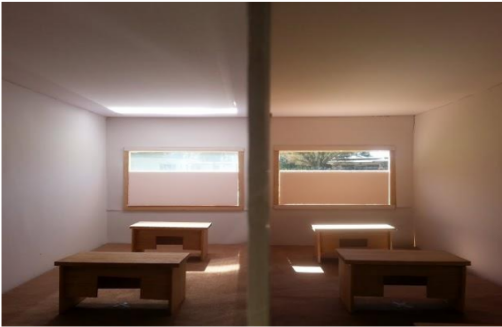
Room with Serralux Daylight Redirecting Film (left) / Room with Standard Glazing (right)
